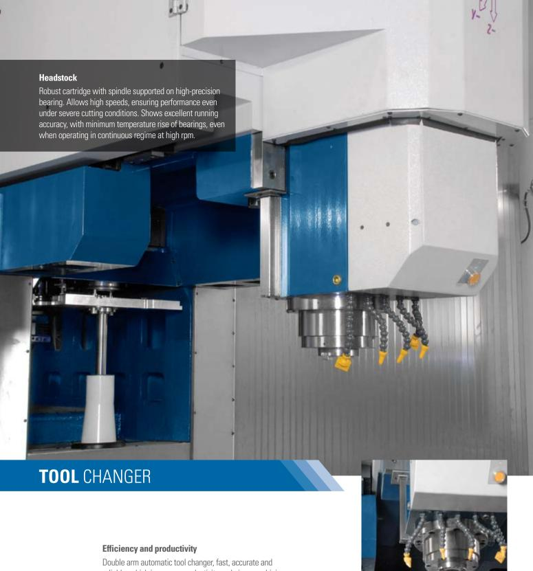
Double arm automatic tool changer, fast, accurate and reliable, which increases productivity and gives machining efficiency.
