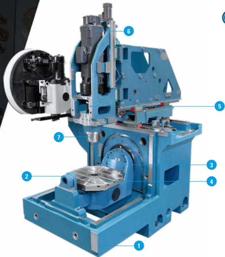
**1 RIGID AND ROBUST MONOBLOCK BASE:** Supports the table assembly, consisting of axes B and C, as well as the cross slide and spindle assembly. The X, Y, and Z axes are equipped with roller linear guides, offering high rigidity, stability, precise positioning, and high-quality surface finish for machining processes, providing maximum efficiency and productivity to the user.
