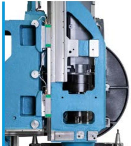
**6 MAIN MOTOR:** Directly coupled to the spindle cartridge, offering high efficiency in torque and power transmission.
