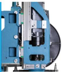
**MAIN MOTOR:** Directly coupled to the spindle cartridge, offering high efficiency in torque and power transmission.
