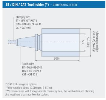
For rotations above 10,000 rpm, it is recommended to use BBT chucks. Regardless of the rotation, all tools should be balanced to G2.5.
